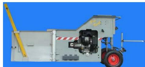
Servicing the reciprocating ram involves two hoses and knocking out two pins – only one bolt is involved! And with the engine slid to the side access is easy.
